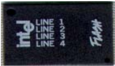
Figure 5. Mark for Pin-1 indicator on 48-Lead 8Mb, 16Mb and 32Mb TSOP
