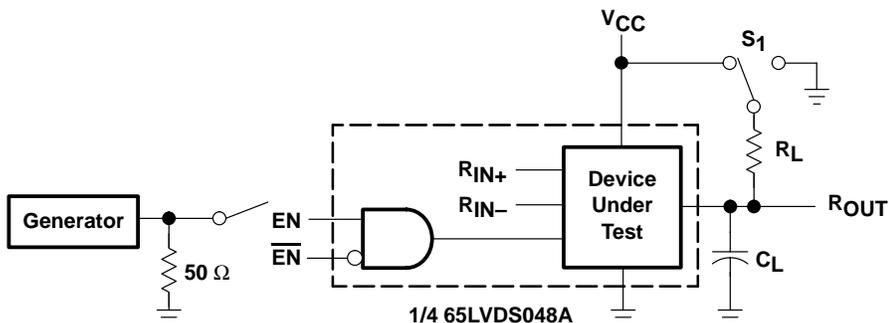
$C_L$  Includes Load and Test Jig Capacitance.
