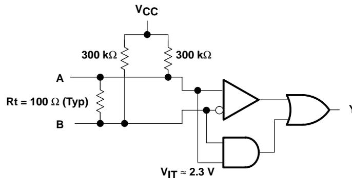
Figure 12. Open-Circuit Fail Safe of the LVDS Receiver
