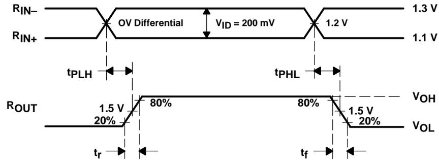
Figure 2. Receiver Propagation Delay and Transition Time Waveforms
