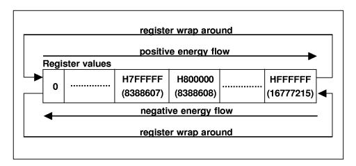
At power-up the register values are underfined and for this reason the msb of the **delta value** (delta value = present register value - previous register value) should be regarded as an indication of the measured energy direction. (0 = positive, 1 = negative).
