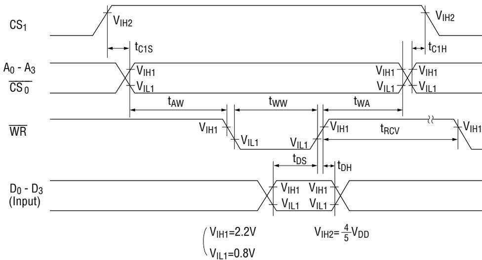
(Note) The ML9070-03 has no  $\overline{CS}_0$  input.
