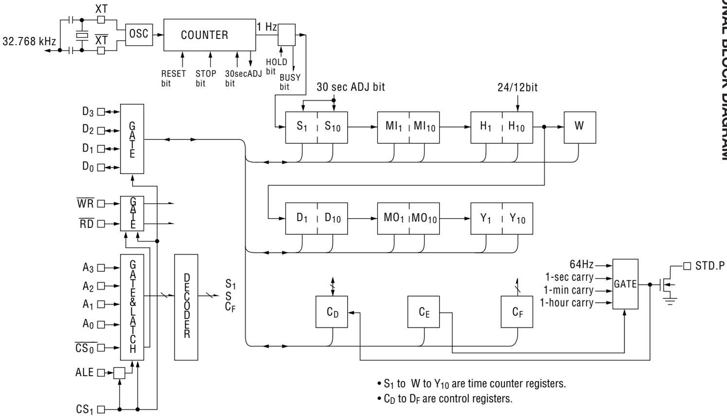
(Note) The ML9070-03 operates similarly as when CS<sub>0</sub> is fixed to "L", and ALE to "H".
