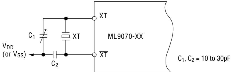
The impedance of the crystal should be less than 30k $\Omega$ .
