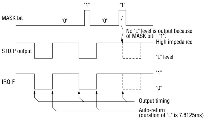
When the IRQ-F bit is read out before auto-return, the IRQ-F bit goes to "0", and the STD.P output keeps "L" level for 7.8125 ms, then goes into the high impedance state.
