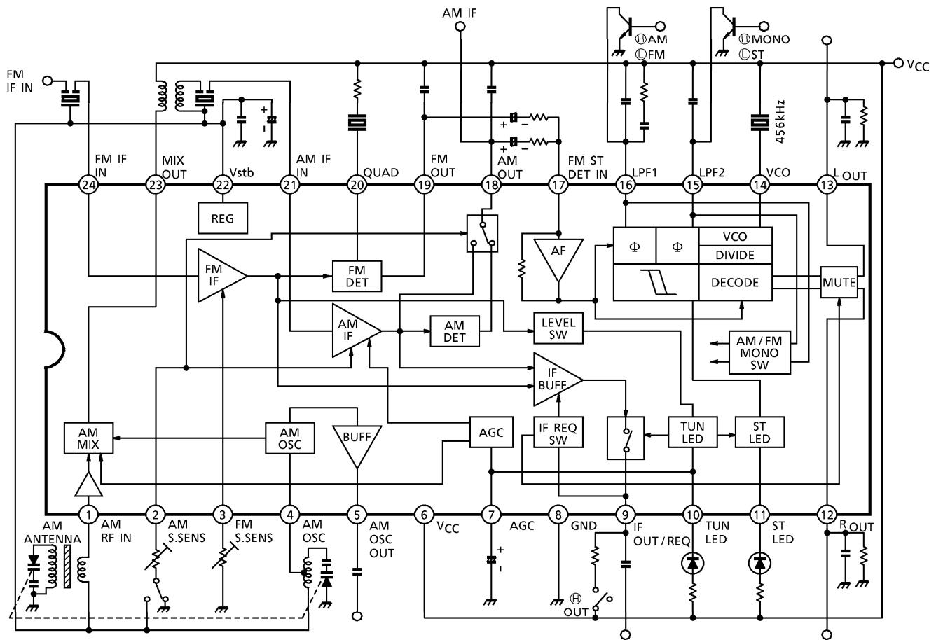
**TERMINAL EXPLANATION** (Terminal Voltage Shows the Typical Value at  $T_a = 25^\circ\text{C}$ ,  $V_{CC} = 5\text{ V}$ ,  $\text{SW}_3 = \text{OFF}$ ,  $\text{SW}_9 = \text{GND}$ , and Non-signal Test Circuit)
