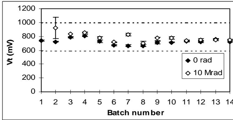
Figure 3. PMOS transistor threshold voltage with dose over production
