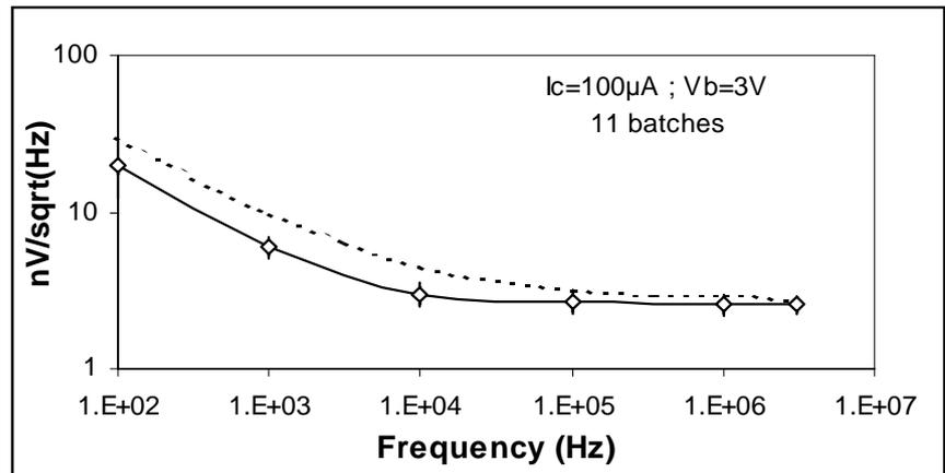
Figure 9. Noise properties of PJFET transistors up to 10 Mrad
