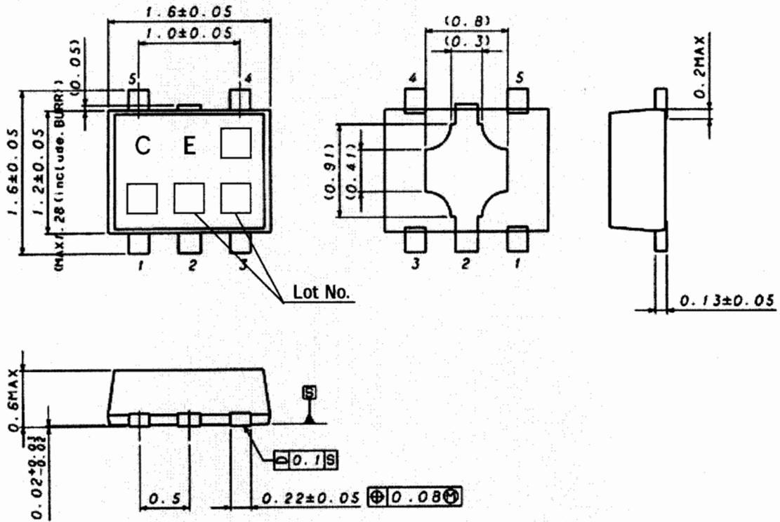
Fig.1 PACKEGE (Plastic Mold) (Unit: mm)
