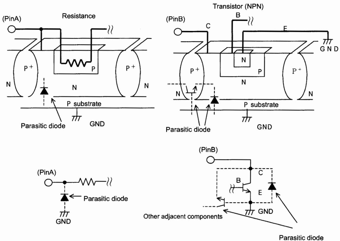
Fig.28 Simplified structure of a Monolithic IC
