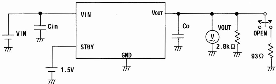
Fig.5 Load excessive response (Characteristic example : Fig.15~17)
