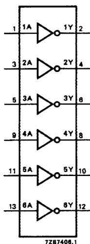
Fig.4 Functional diagram.
