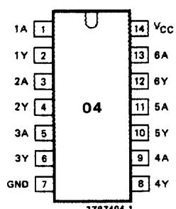
Fig.1 Pin configuration.
