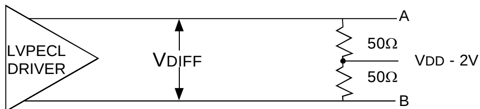
Test Circuit for LVPECL Output Characteristics
