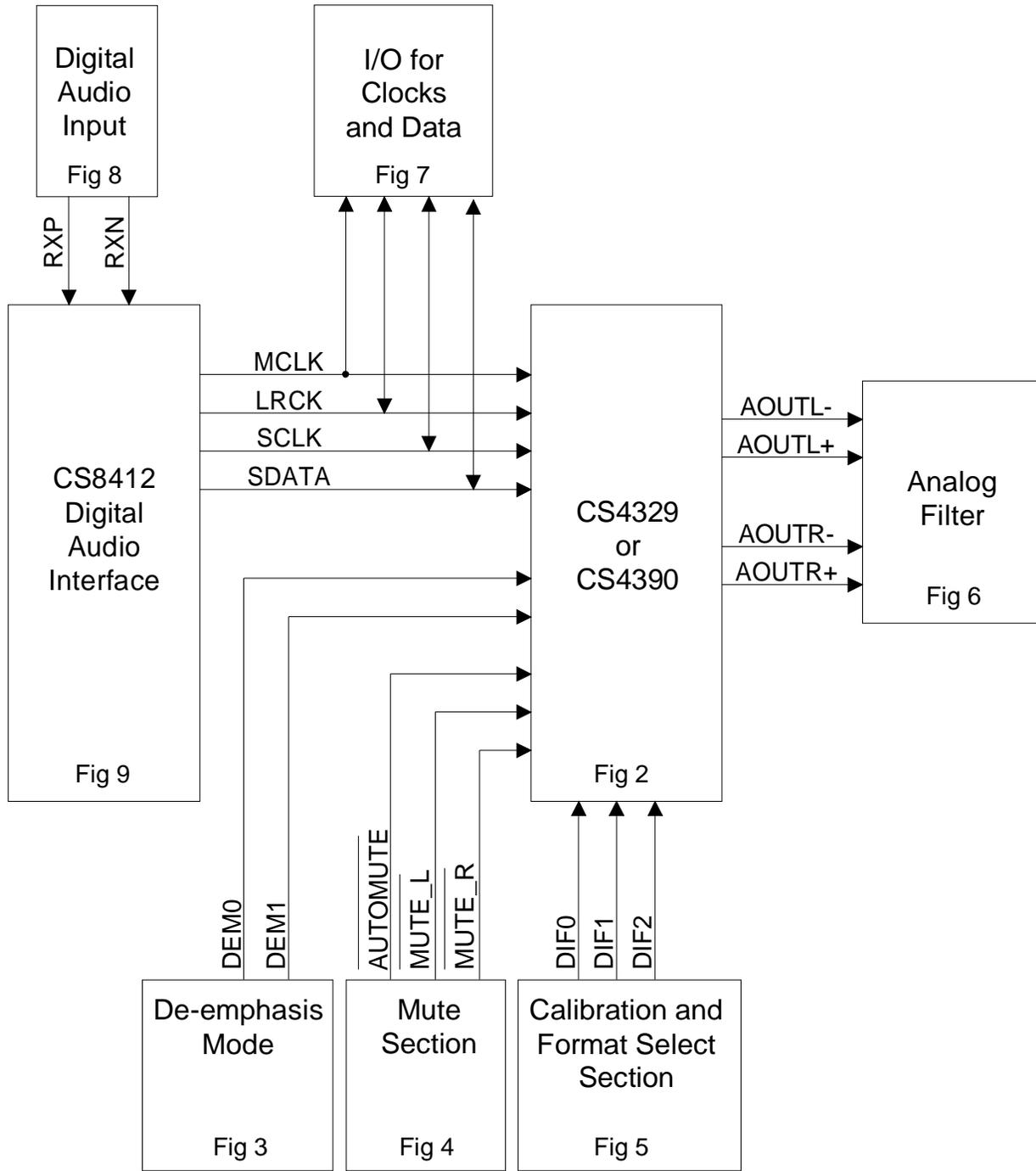
**Figure 1. System Block Diagram and Signal Flow**
