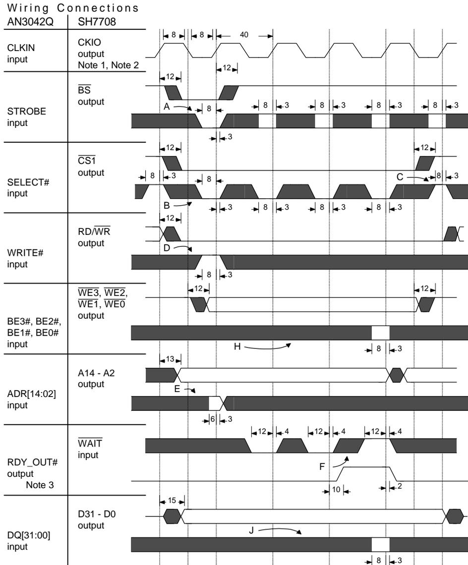
INPUT WAVEFORMS REPRESENT SIGNAL INPUT REQUIREMENTS.
