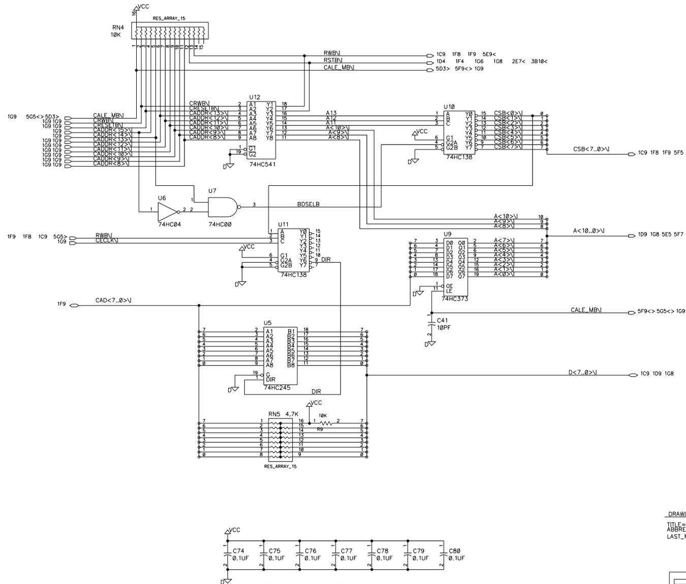
DECOUPLING CAPS FOR DECODING LOGIC
