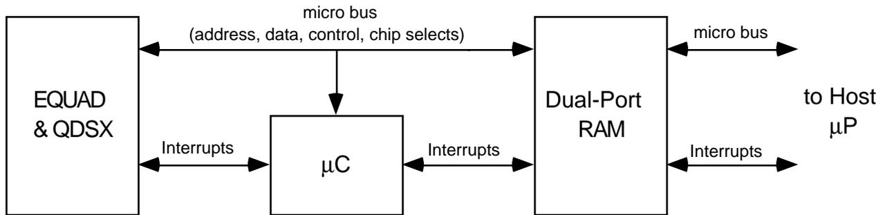
Subroutines are required to operate dedicated I/O pins as the micro bus during external accesses. Since the interrupt service routines will alternate between accessing the EQUAD, QDSX and the dual-port RAM, it saves instruction cycles to have separate subroutines dedicated to each, where the address would be taken from different pre-defined registers.
