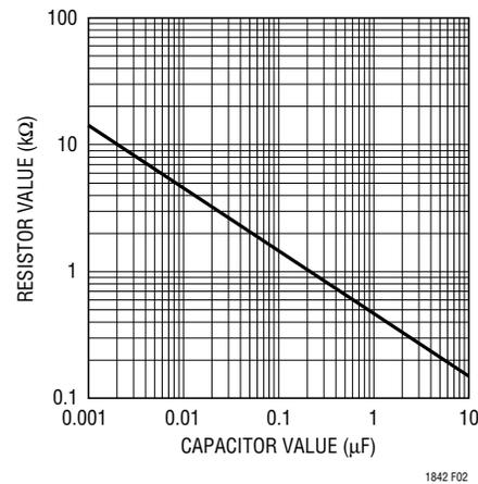
Figure 2. Damping Resistance vs Bypass Capacitor Value
