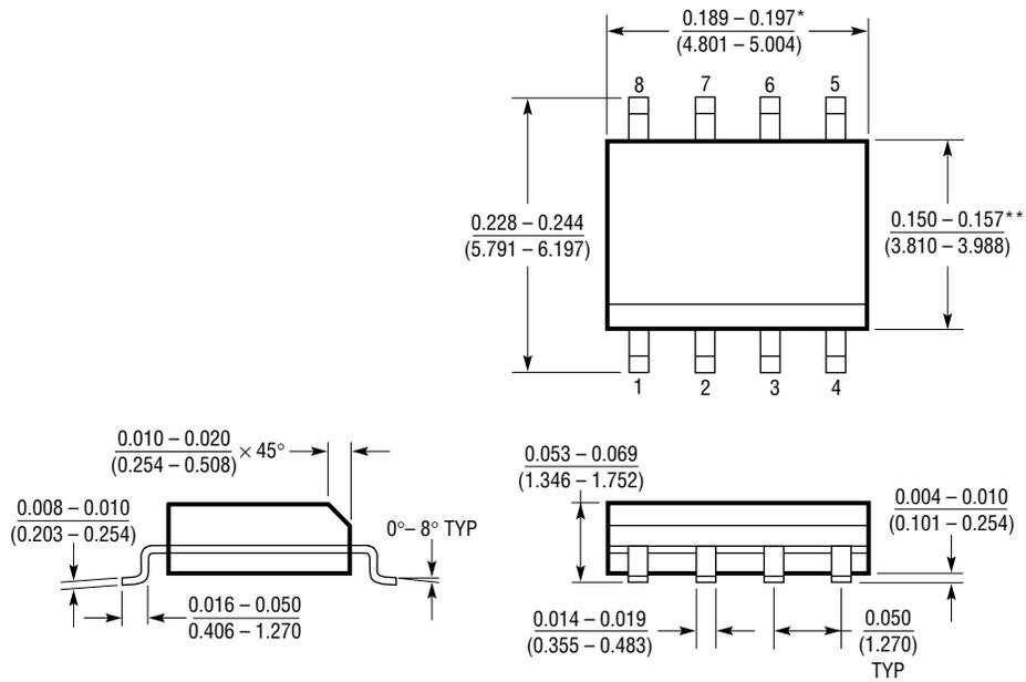
\*DIMENSION DOES NOT INCLUDE MOLD FLASH. MOLD FLASH SHALL NOT EXCEED 0.006" (0.152mm) PER SIDE
