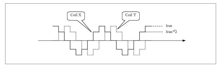
Whereas the figure below shows the current fed to one coil in 1/16th microstepping (1 electrical period).
