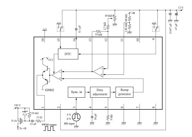
Note) When both of the pin 4 and the pin 5 are open, minimum pulse width of PWM output is 2.0  $\mu s.$
