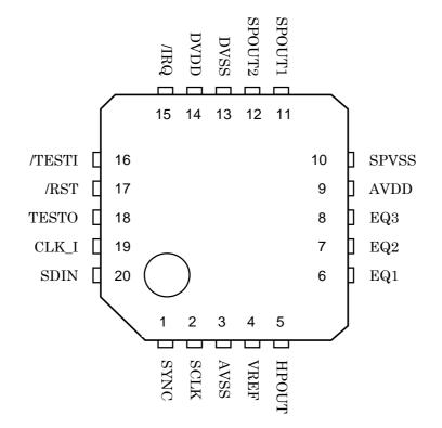
20 Pin QFN Top View
