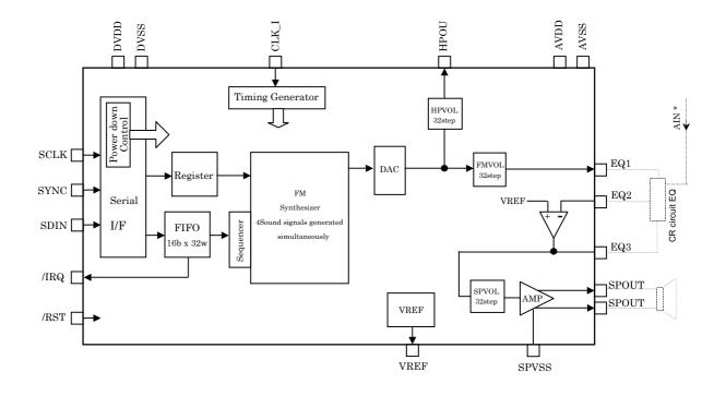
Concerning AIN signal inputted into equalizer circuit
