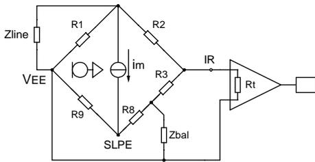
Fig 4 Equivalent circuit of UTC1062A anti-sidetone bridge
