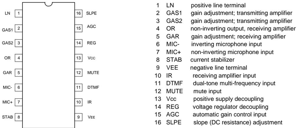
Fig.2 Pining Diagram
