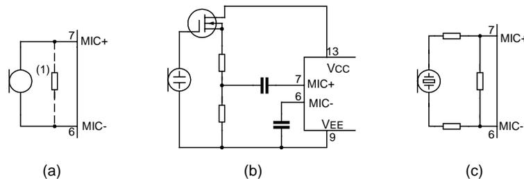
(a) Magnetic or dynamic microphone. The resistor marked (1) may be connected to decrease the terminating impedance.
