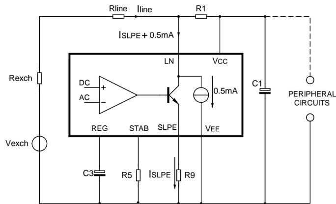
Fig.8 Supply arrangement
