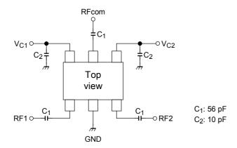
The values of capacitors depends on the application frequency range and the board pattern layout.
