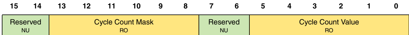
Figure 3-129. CCFnR, CC Part Buffer of a Double Transmit Message Buffer Filter Registers
