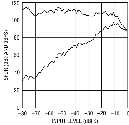
LTC2207-14: SFDR vs Input Level, f_{IN} = 140.1\text{MHz} , PGA = 1, RAND "On", Dither "Off"
