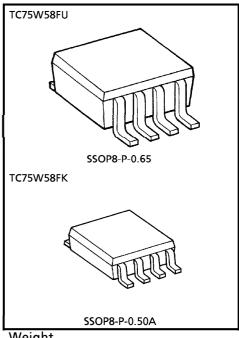
Weight SSOP8-P-0.65 : 0.021g (Typ.) SSOP8-P-0.50A : 0.01g (Typ.)
