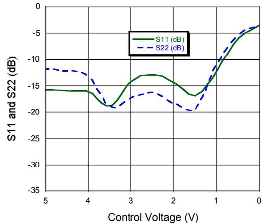
**Return Loss vs. Control Voltage, F = 2200 MHz**
