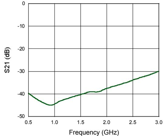
**Voltage Variable Absorptive Attenuator
