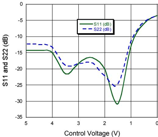
**Return Loss vs. Control Voltage, F = 1800 MHz**
