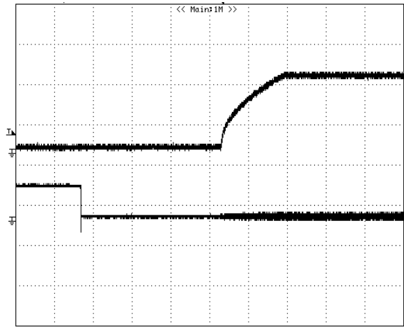
Figure 5: Turn-on transient at full rated load current (constant current load) (2 ms/div). V_{in}=48V . Top Trace: V_{out} , 1V/div; Bottom Trace: ON/OFF input, 5V/div
