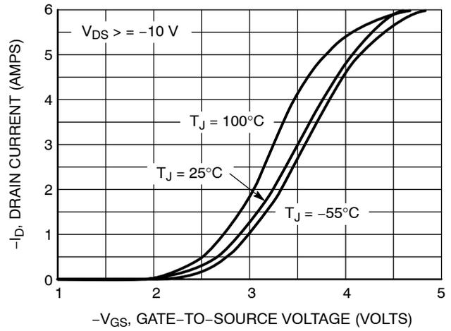
Figure 2. Transfer Characteristics
