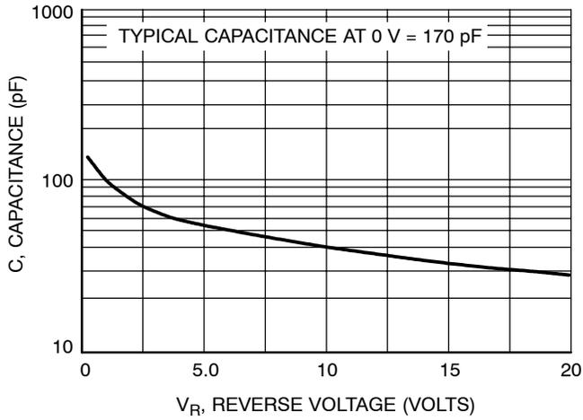
Figure 19. Typical Capacitance
