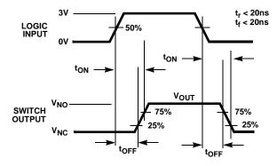
Logic input waveform is inverted for switches that have the opposite logic sense.
