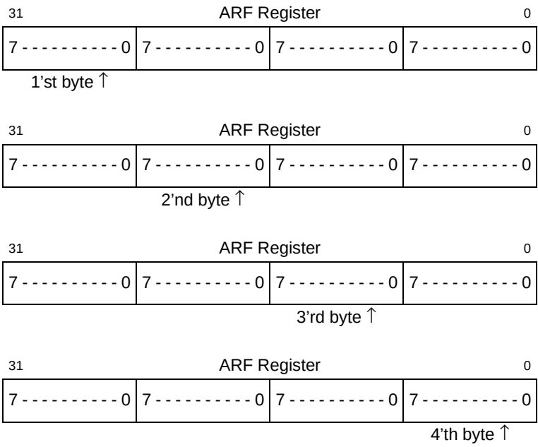
Figure 5-3-9 Register Operation (ARF) for 8-Bit Width DMA Access
