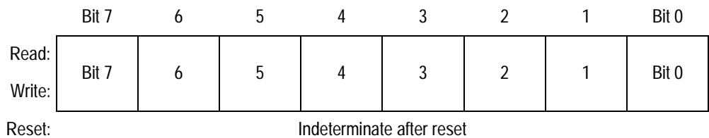
Figure 10-15. TIM Channel 1 Register Low (TCH1L)
