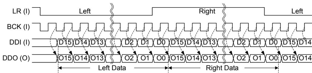
During playback, the 16-bit playback data is input serially from the MSB to the DDI pin in synchronization with the clock signal of the BCK pin. The DDI pin input data is taken in the LSI at the rising edge of the BCK clock signal. The recording data is output from the DDO pin at the falling edge of the BCK clock signal during recording.
