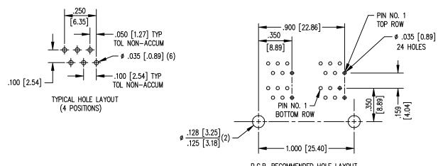
P.C.B. RECOMMENDED HOLE LAYOUT SEEN FROM COMPONENT SIDE TOLERANCE ±.003 [0.08] UNLESS OTHERWISE SPECIFIED
