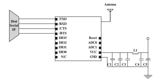
Parts List for XE900SL10 Typical Connection Diagram
