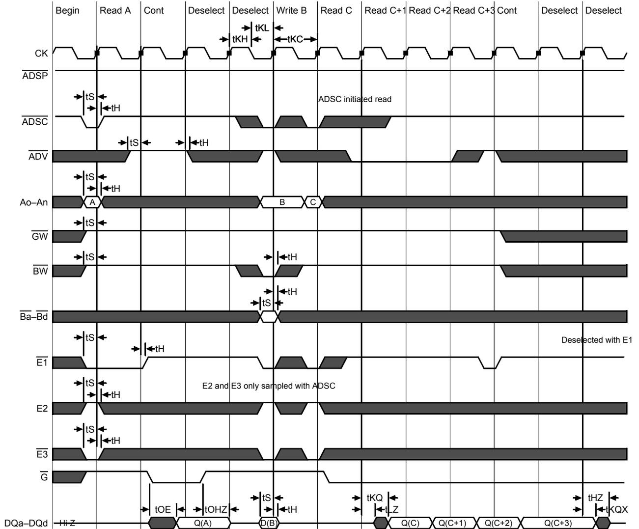
Flow Through Mode Timing (DCD)
