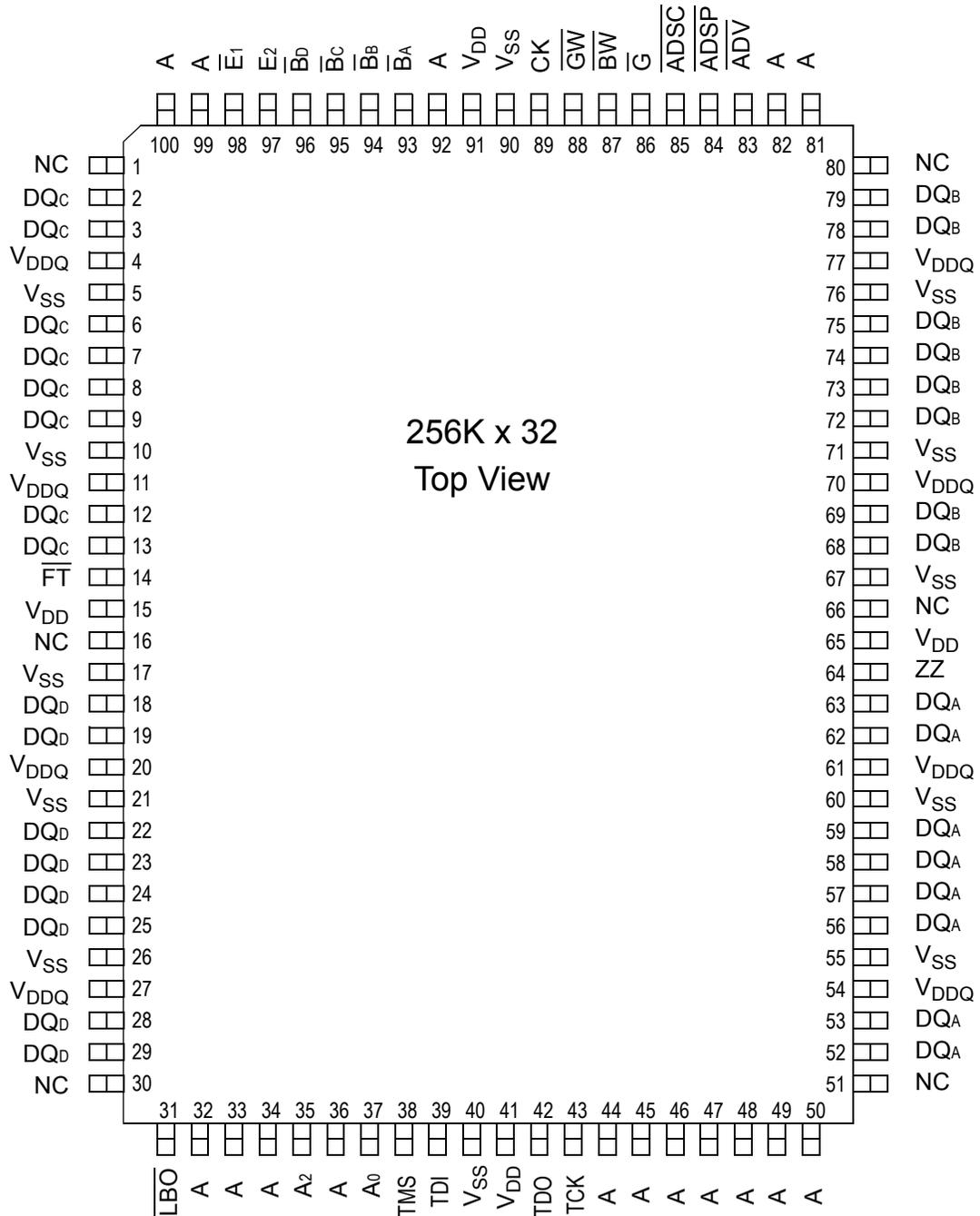
GS881E36B 100-Pin TQFP Pinout (Package T)
