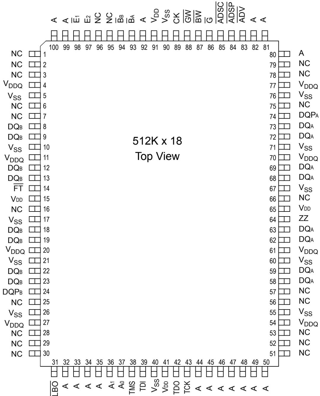
GS881E32B 100-Pin TQFP Pinout (Package T)
