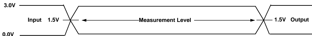
Figure 17. Input Waveforms and Measurement Levels
