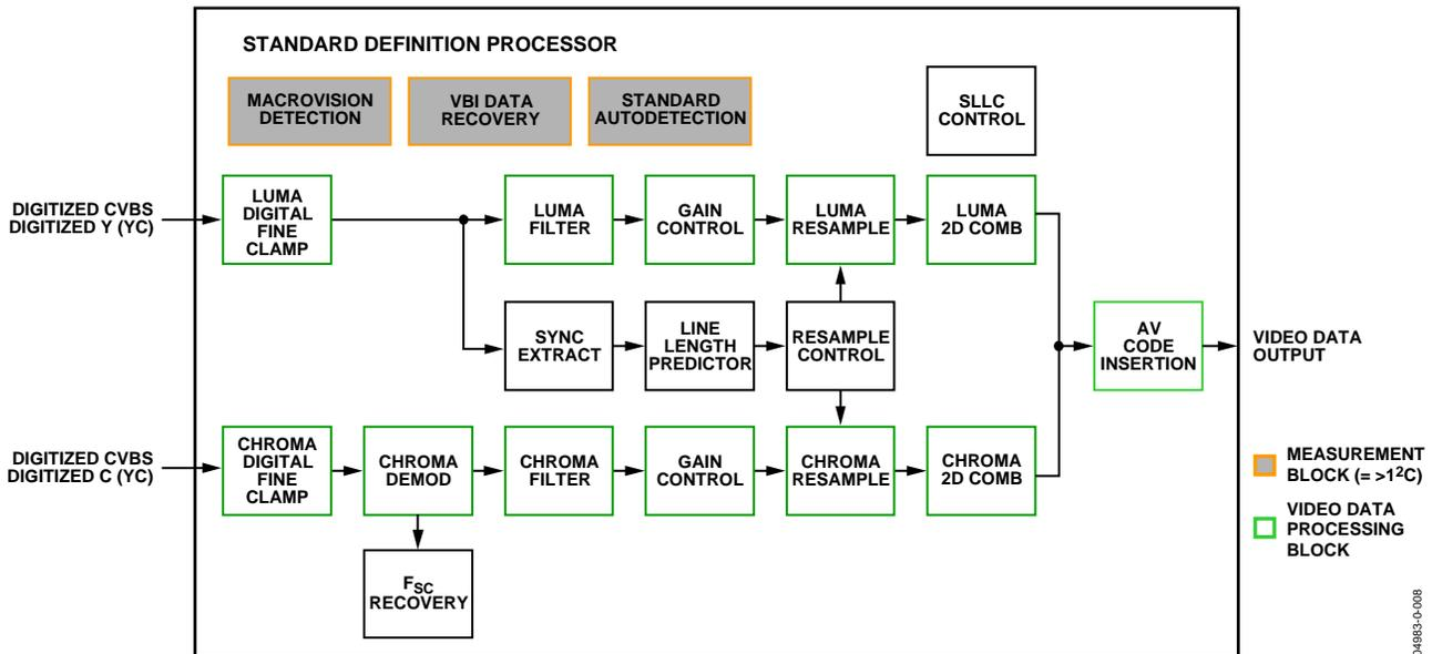
Figure 8. Block Diagram of the Standard Definition Processor
