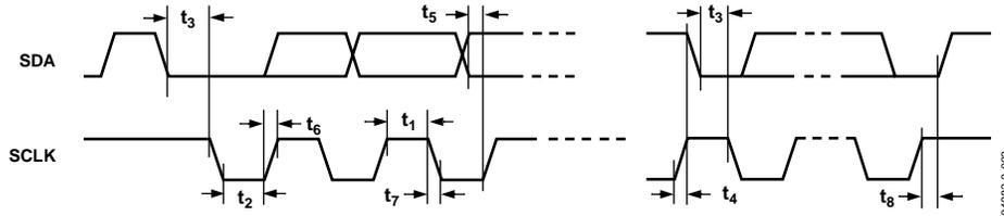
Figure 2. I<sup>2</sup>C Timing
