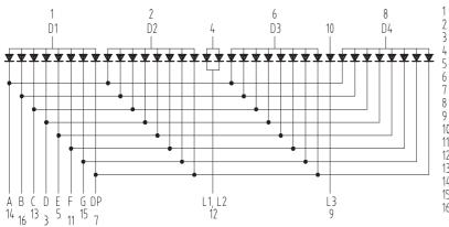
Common Anode 1 Common Anode D1 2 Common Anode D2 3 Cathode D 4 Anode L1, L2 5 Cathode É 6 Common Anode D3 7 Cathode DP 8 Common Anode D4 9 Cathode L3 10 Anode L3 11 Cathode F 12 Cathode L1, L2 13 Cathode C 14 Cathode A 15 Cathode G 16 Cathode B
