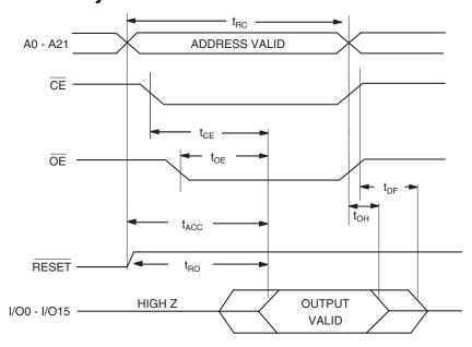
Notes: 1.  $\overline{\text{CE}}$  may be delayed up to  $t_{\text{ACC}}$  -  $t_{\text{CE}}$  after the address transition without impact on  $t_{\text{ACC}}$ .
