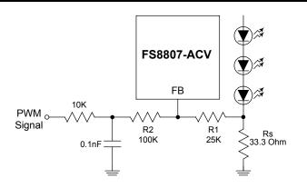
4. Using a Logic Signal
