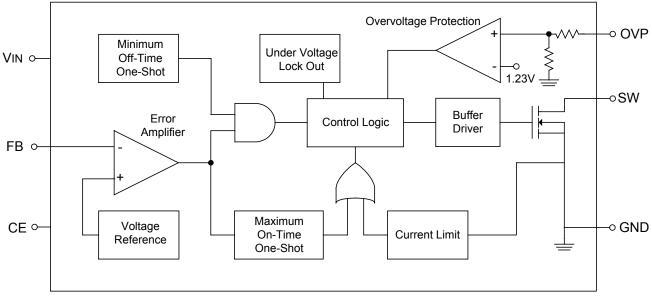
Fig 2. FS8807 Simplified Functional Block Diagram
