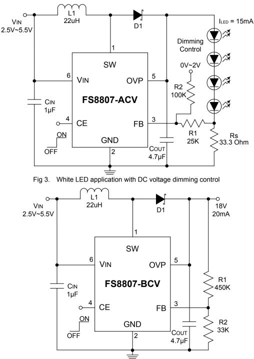
Fig 4. Typical 18V application for line drivers or LCD bias
