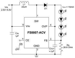
Fig 1. FS8807 Typical Application for driving 4 White LEDS
