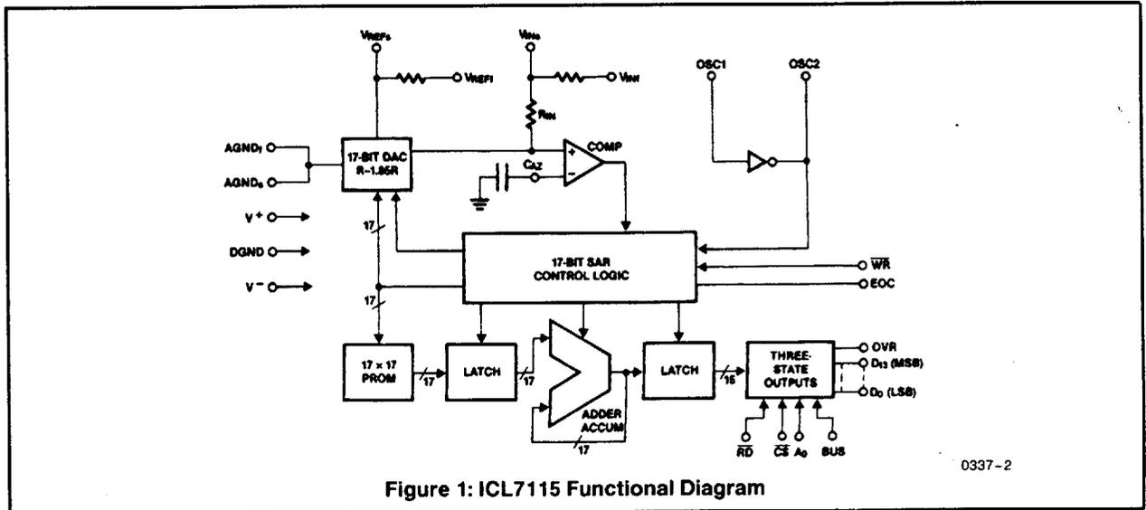
Figure 1: ICL7115 Functional Diagram
