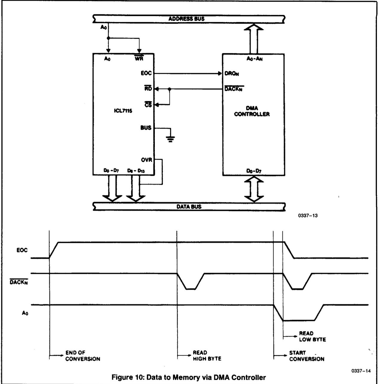
Figure 10: Data to Memory via DMA Controller
