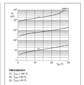
Fig.6 Reverse current as a function of reverse
