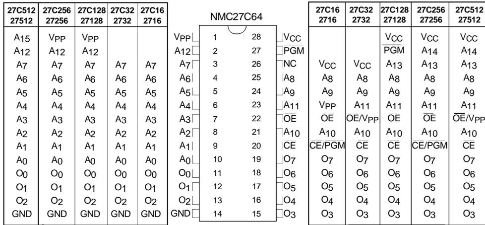
**Note:** Socket compatible EPROM pin configurations are shown in the blocks adjacent to the NMC27C64 pins.
