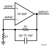
Figure 1. Compensation for Feedback Node Capacitance
