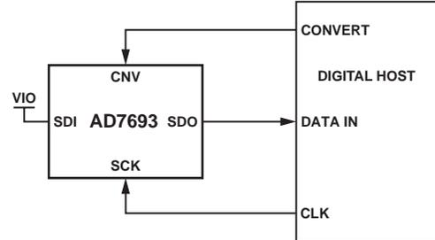
Figure 18.  $\overline{\text{CS}}$  Mode 3-Wire, No BUSY Indicator Connection Diagram (SDI High)
