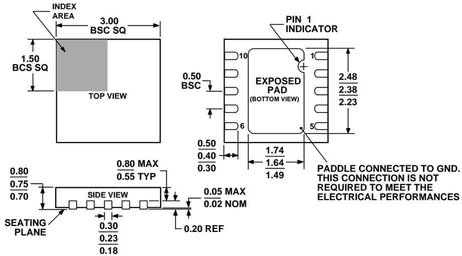
Figure 33. 10-Lead Lead Frame Chip Scale Package [QFN (LFCSP\_WD)]
