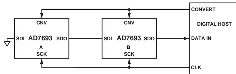
Figure 26. Chain Mode, No BUSY Indicator Connection Diagram
