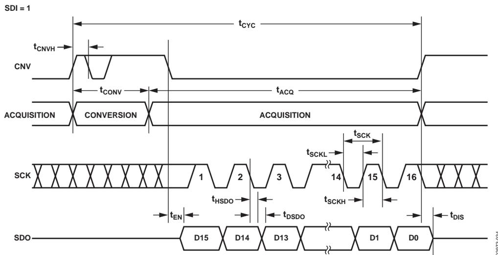
Figure 19.  $\overline{\text{CS}}$  Mode 3-Wire, No BUSY Indicator Serial Interface Timing (SDI High)
