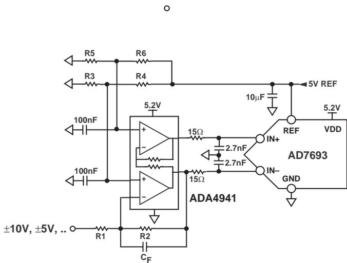
Figure 17. Single-Ended-to-Differential Driver Circuit
