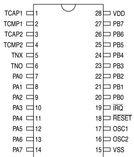
**Figure 11-3** 28-pin PDIP/SOIC pinout
