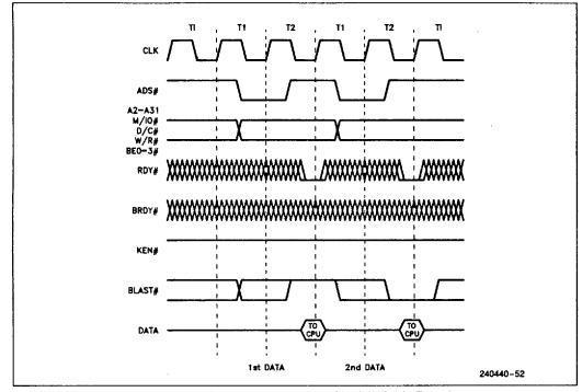
Figure 7.9. Non-Cacheable, Non-Burst, Multiple Cycle Transfers
