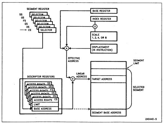
Figure 2.17. Addressing Mode Calculations
