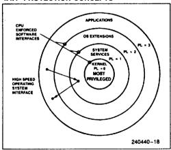
Figure 4.14. Four-Level Hierarchical Protection
