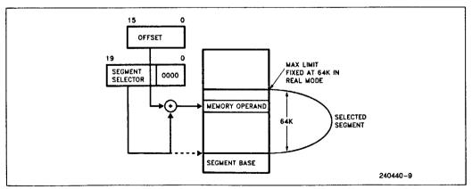
Figure 3.1. Real Address Mode Addressing
