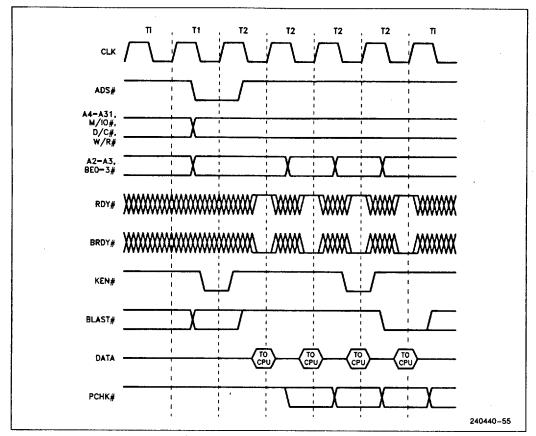
Figure 7.12. Burst Cacheable Cycle
