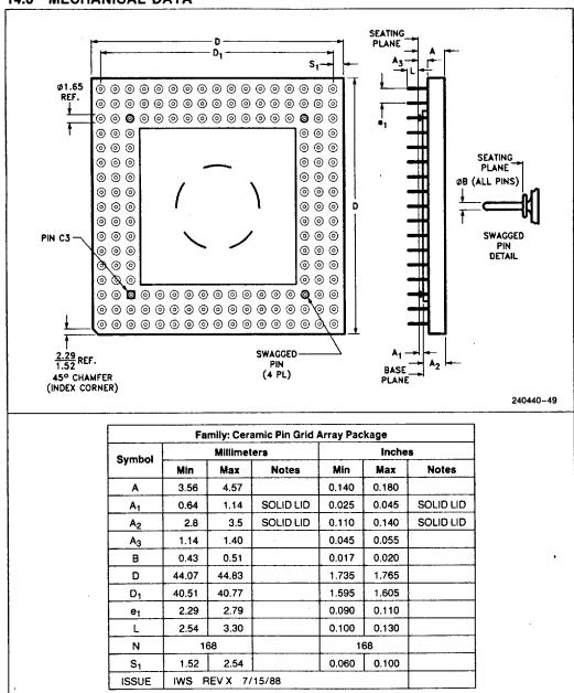
Figure 14.1. 168 Lead Ceramic PGA Package Dimensions
