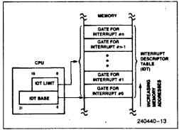
Figure 4.4. Interrupt Descriptor Table Register Use
