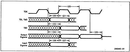
Figure 13.7. Test Signal Timing Diagram
