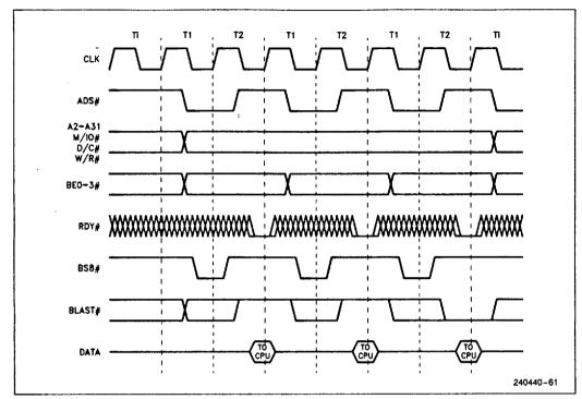
Figure 7.18. 8-Bit Bus Size Cycle
