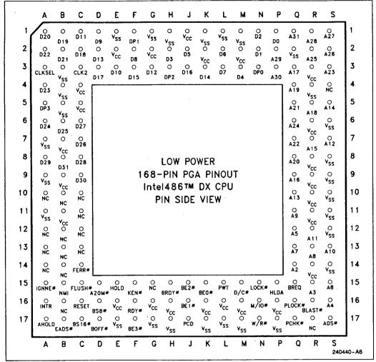
Figure 15.2. Low Power Intel486™ DX CPU Pinout (Pin Side View)
