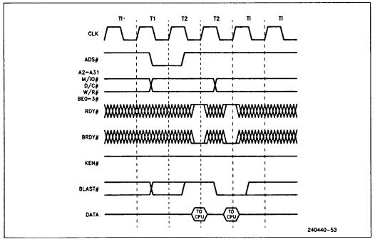
Figure 7.10. Non-Cacheable Burst Cycle
