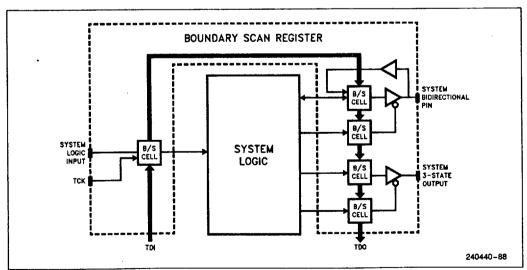
Figure 8.5. Logical Structure of Boundary Scan Register
