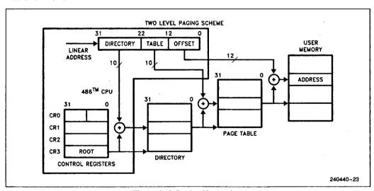
Figure 4.19. Paging Mechanism
