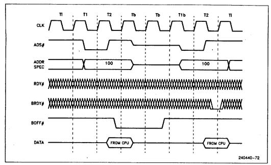
Figure 7.29. Restarted Write Cycle
