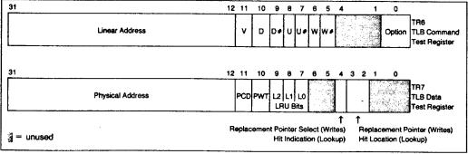
Figure 8.4. TLB Test Registers
