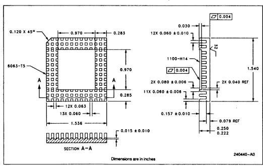
Figure 12.4. Intel OverDrive™ Processor Heat Sink Dimensions
