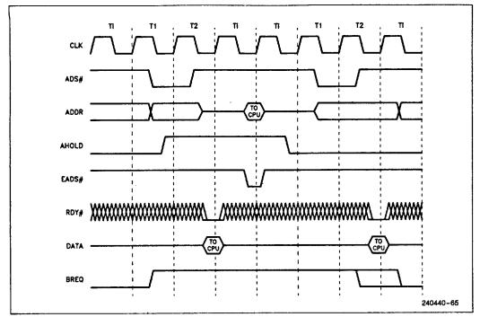
Figure 7.22. Fast Internal Cache Invalidation Cycle
