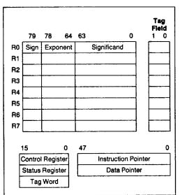
Figure 2.7. Floating Point Registers
