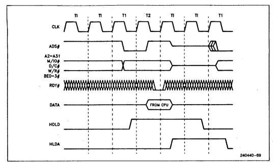
Figure 7.26a. HOLD/HLDA Cycles
