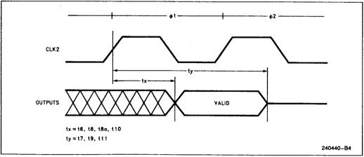
Figure 15.10. Valid and Float Delay Timings
