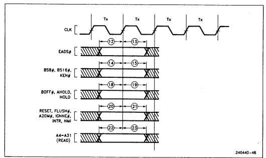
Figure 13.2. Input Setup and Hold Timing
