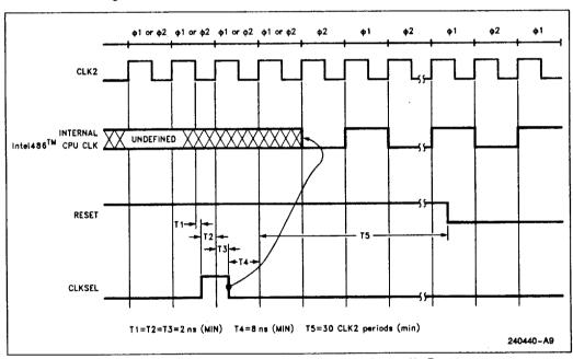
Figure 15.5. CLKSEL Timing Definition during Power-Up Reset
