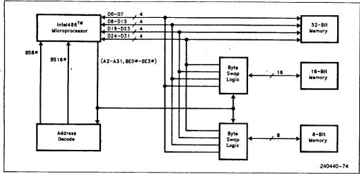
Figure 7.6. Data Bus Interface to 16- and 8-bit Memories
