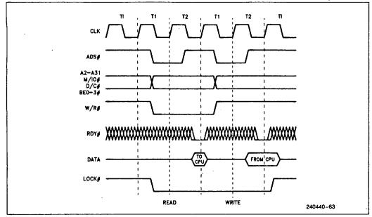
Figure 7.20. Locked Bus Cycle
