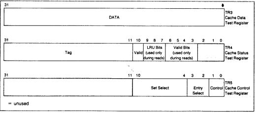
Figure 8.1. Cache Test Registers
