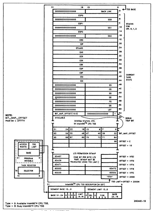
Figure 4.15a. Intel486™ Microprocessor TSS and TSS Registers
