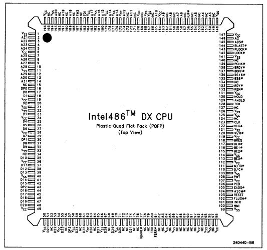
Figure 1.5. Intel486TM DX CPU 196 Lead PQFP Pinout
