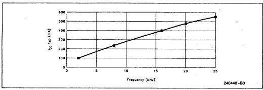
Figure 15.6. Frequency vs I<sub>CC</sub>(typ) (PGA Version)
