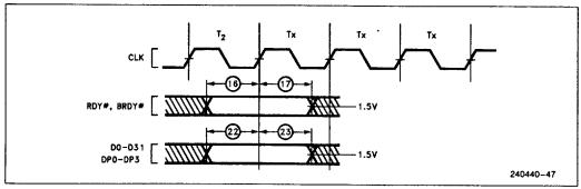
Figure 13.3. Input Setup and Hold Timing
