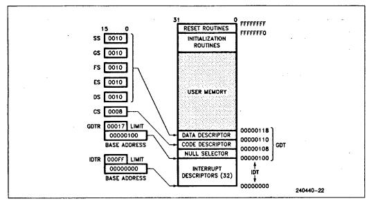
Figure 4.17. Simple Protected System
