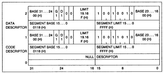
Figure 4.18. GDT Descriptors for Simple System
