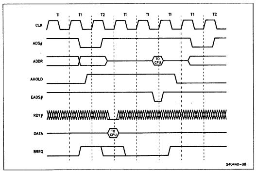
Figure 7.23. Typical Internal Cache invalidation Cycle
