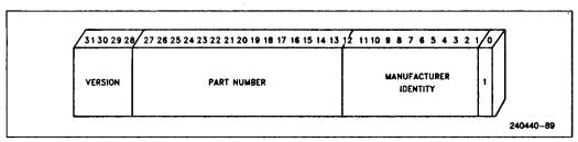
Figure 8.6. Format of Device Identification Register
