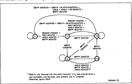
Figure 7.30. Bus State Diagram
