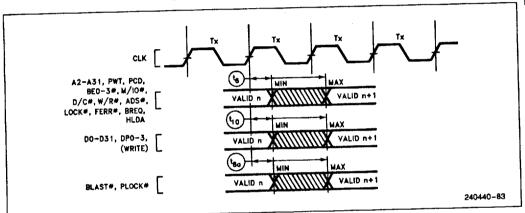
Figure 13.5. Output Valid Delay Timing
