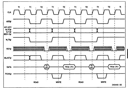
Figure 7.7. Basic 2-2 Bus Cycle
