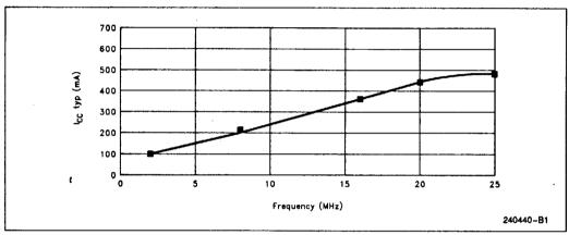
Figure 15.7. Frequency vs I<sub>CC</sub>(typ) (PQFP Version)
