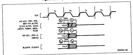
Figure 13.6. Maximum Float Delay Timing
