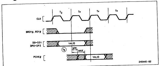
Figure 13.4. PCHK # Valid Delay Timing
