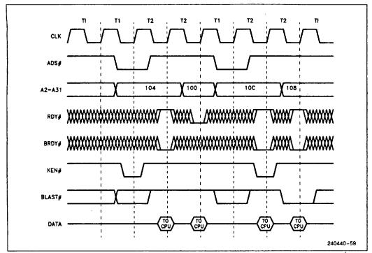
Figure 7.16. Interrupted Burst Cycle
