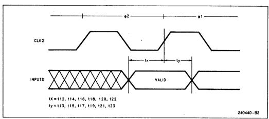
Figure 15.9. Setup and Hold Timings
