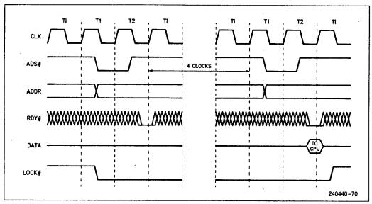
Figure 7.27. Interrupt Acknowledge Cycles
