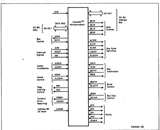
Figure 6.1. Functional Signal Groupings
