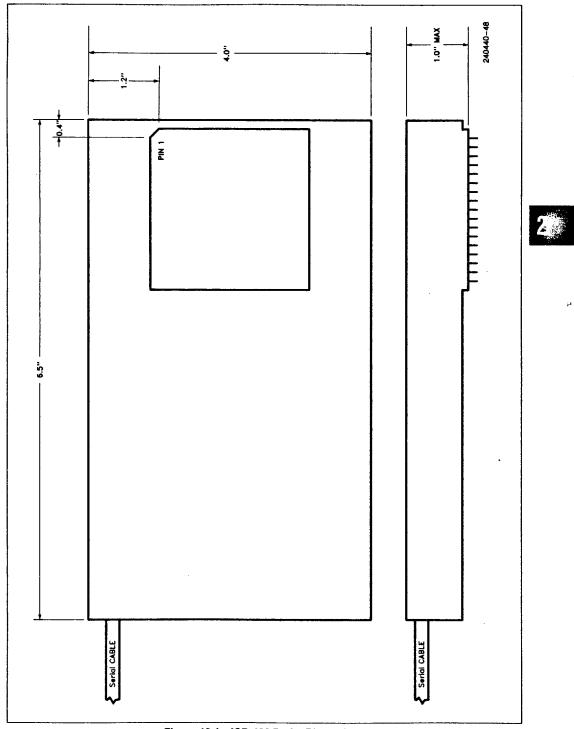
Figure 13.4a. ICD-486 Probe Dimensions
