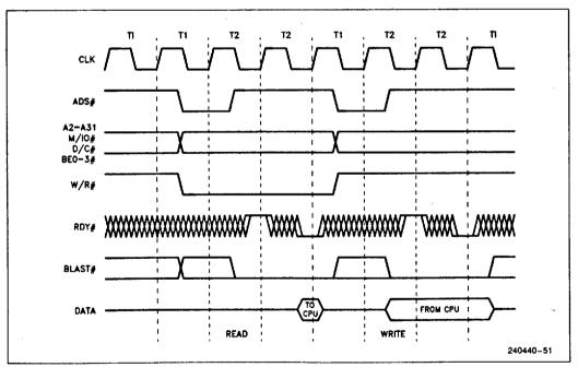
Figure 7.8. Basic 3-3 Bus Cycle
