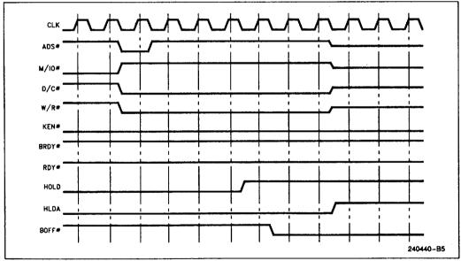
Figure 7.26b. HOLD Request Acknowledged during BOFF#
