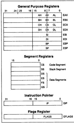
Figure 2.1. Base Architecture Registers
