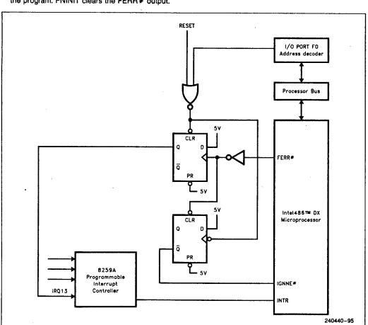
Figure 7.31. DOS Compatible Numerics Error Circuit
