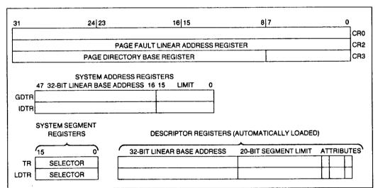
Figure 2.4. System Level Registers
