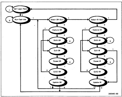
Figure 8.7. TAP Controller State Diagram
