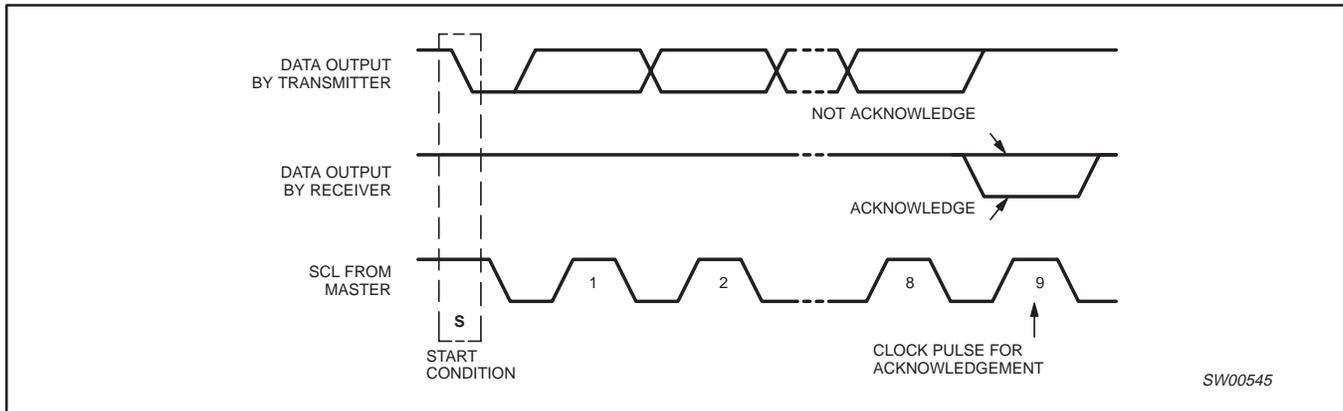
Figure 6. Acknowledgment on the I<sup>2</sup>C-bus
