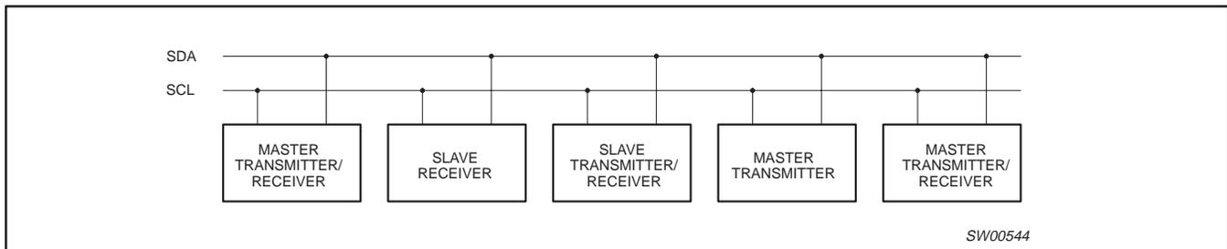
Figure 5. System configuration
