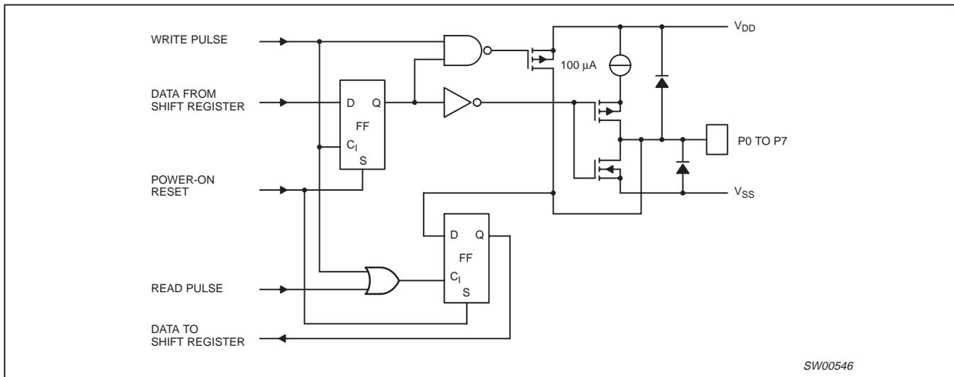
Figure 7. Simplified schematic diagram of each I/O
