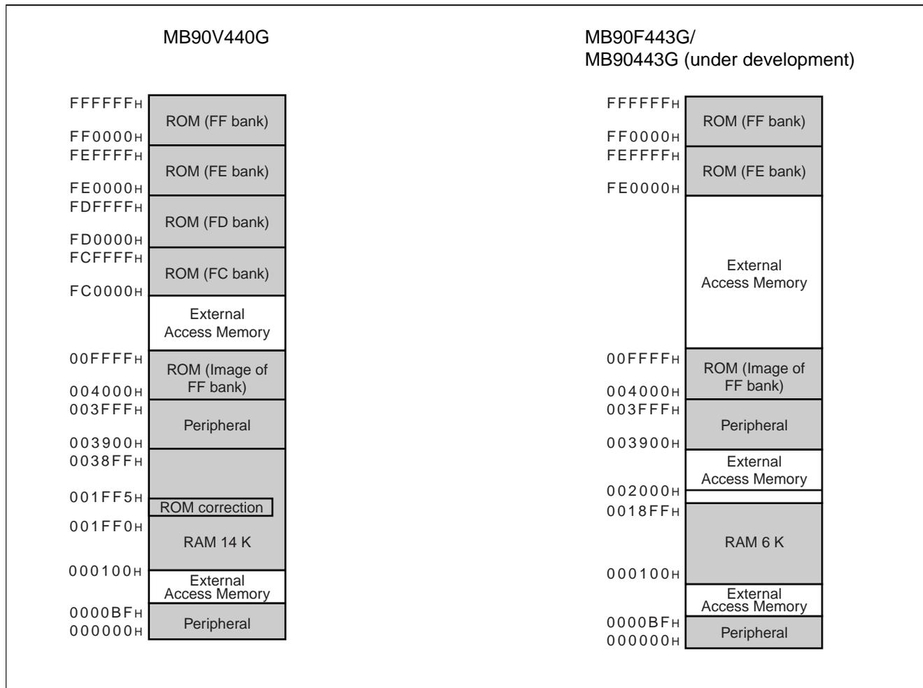
Note : The high-order portion of bank 00 gives the image of the FF bank ROM to make the small model of the C compiler effective. Since the low-order 16 bits are the same address, the table in ROM can be referenced without using the far specification in the pointer declaration.
