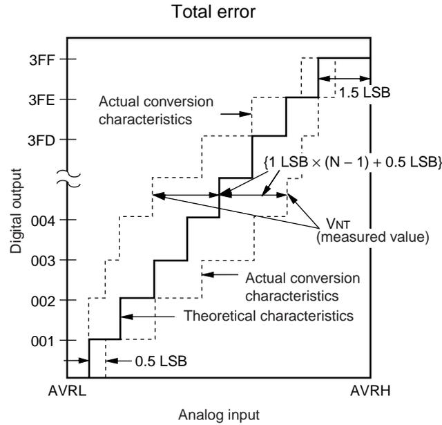
$$\text{Total error of digital output } N = \frac{V_{NT} - \{1 \text{ LSB} \times (N - 1) + 0.5 \text{ LSB}\}}{1 \text{ LSB}} \text{ [LSB]}$$
