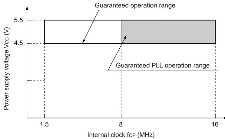
Relationship between oscillation frequency and internal operating clock frequency
