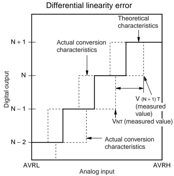
$$\text{Linearity error of digital output } N = \frac{V_{NT} - \{1 \text{ LSB} \times (N - 1) + V_{OT}\}}{1 \text{ LSB}} \text{ [LSB]}$$
