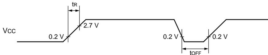
Sudden changes in the power supply voltage may cause a power on reset. We recommend to raise the voltage smoothly to suppress fluctuation during operation, as shown in the figure below. Perform while not using the PLL clock. However, if voltage drops are within 1 V/s, you can operate while using the PLL clock.
