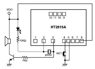
\* The IC substrate should be connected to VDD in the PCB layout artwork.
