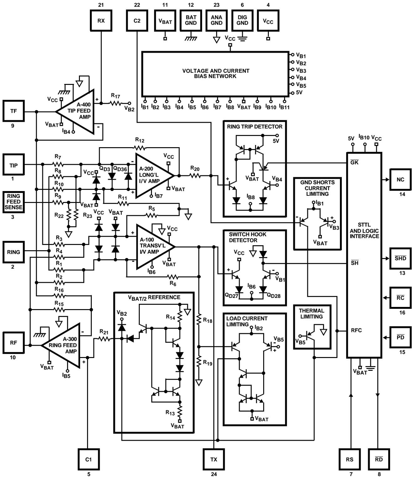
FIGURE 8. FUNCTIONAL SCHEMATIC
