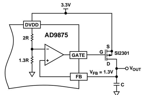
Figure 3b. Connections for a 1.3 V Linear Regulator
