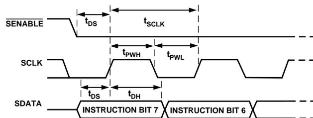
Figure 8. Timing Diagram Register Write to AD9875/AD9876
