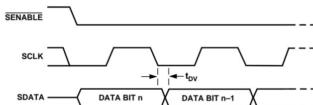
Figure 9. Timing Diagram Register Read from AD9875/AD9876
