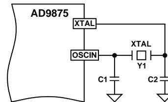
Figure 3a. Connections for Fundamental Mode Crystal
