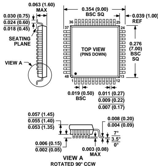
CONTROLLING DIMENSIONS ARE IN MILLIMETERS.
