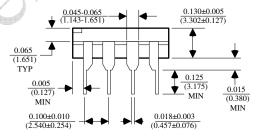
\*DIMENSIONS DO NOT INCLUDE MOLD FLASH OR PROTUSIONS. MOLD FLASH OR PROTUSIONS SHALL NOT EXCEED 0.010" (0.254mm)
