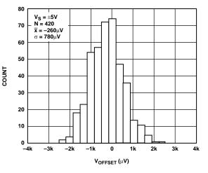
Figure 33. Input Offset Voltage Distribution
