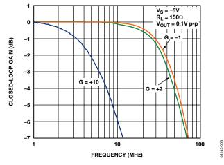
Figure 4. Small Signal Frequency Response for Various Gains
