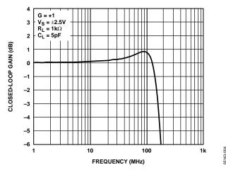
Figure 2. Small Signal Frequency Response
