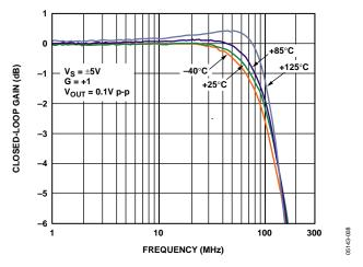
Figure 8. Small Signal Frequency Response for Various Temperatures
