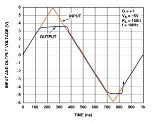
Figure 18. Input Overdrive Recovery
