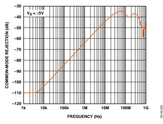
Figure 34. Common-Mode Rejection Ratio (CMRR) vs. Frequency
