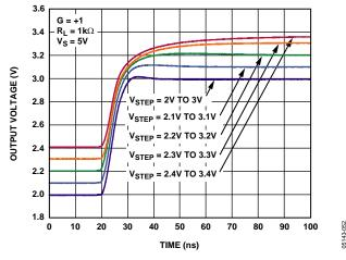
Figure 38. Output Rising Edge for 1 V Step at Input Headroom Limits
