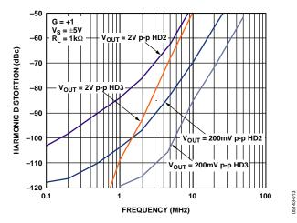
Figure 16. Harmonic Distortion vs. Frequency for Various VOUT
