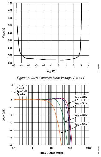
Figure 37. Unity-Gain Follower Bandwidth vs. Input Common-Mode
