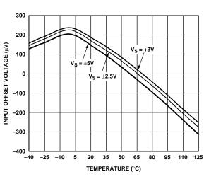
Figure 27. Input Offset Voltage vs. Temperature for Various Supplies
