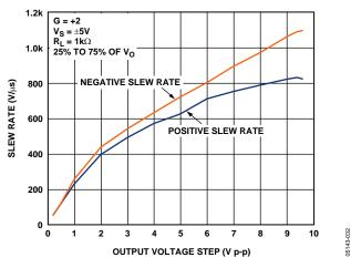
Figure 24. Slew Rate vs. Output Voltage
