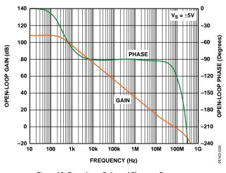
Figure 12. Open-Loop Gain and Phase vs. Frequency
