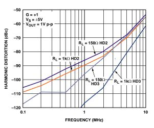
Figure 15. Harmonic Distortion vs. Frequency for Various Loads
