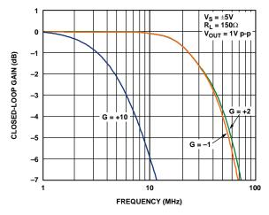
Figure 9. Large Signal Frequency Response for Various Gains
