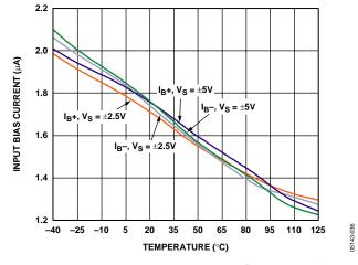
Figure 28. Input Bias Current vs. Temperature for Various Supplies
