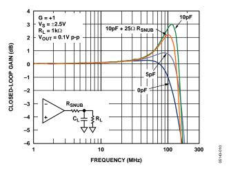
Figure 7. Small Signal Frequency Response for Various Capacitor Loads
